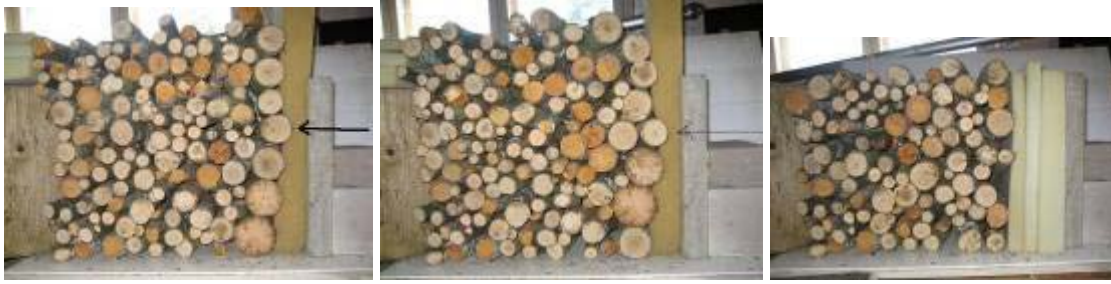
Figure 2.2.5. Model tests that imply that the centre of impact of the slide triangle is roughly at half the height of the stow.
