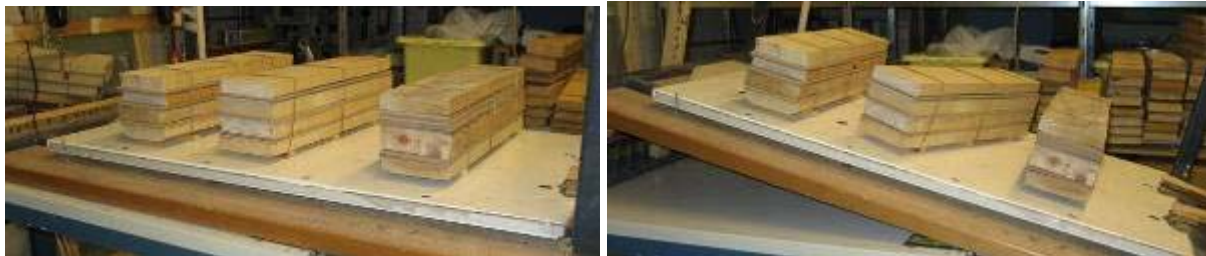
Figure 3.1.2 a,b,c) Friction tests with model timber packages.
