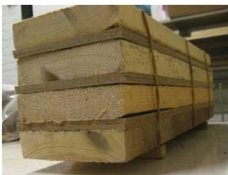
Figure 3.1.1 a) An x-model package b) another x-package deformed. c) A y-model package, “soft version” with masonite and rubber bands. d) y-package deformed.
