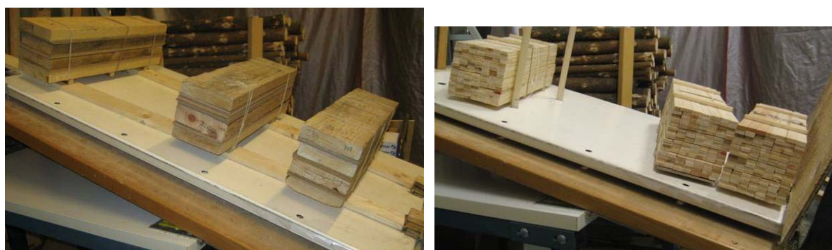
Figure 3.1.3 a) Friction test with y-packages on wooden slats b) x-packages on the model hatch surface.
