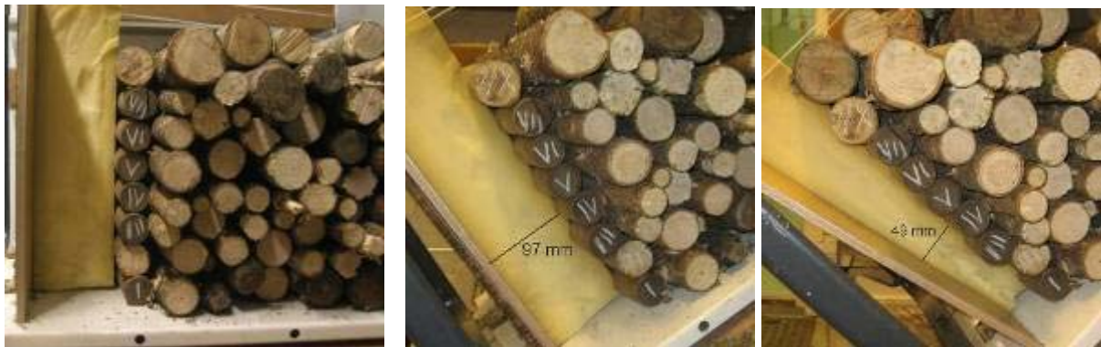
Figure 2.2.6 Force distribution tests at 0, 33 and 49 degrees with an example of difference in distance.
