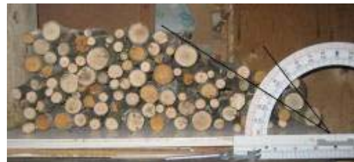
Test nr 7: The slide angle is 41^\circ to 60^\circ from the vertical line
