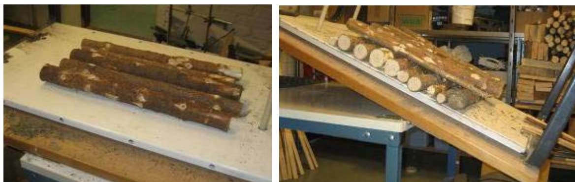
Figure 2.2.1. Friction tests with a) longitudinally and b) transversally placed logs.
