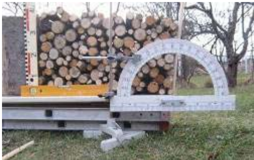
Test nr 3: The slide angle is 51^\circ from the vertical line.
