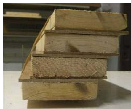
Figure 3.1.1 a) An x-model package b) another x-package deformed. c) A y-model package, “soft version” with masonite and rubber bands. d) y-package deformed.
