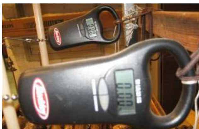
Figure 2.1.3 Dynamometers displaying tension in kilograms ranging up to 23 kg.
