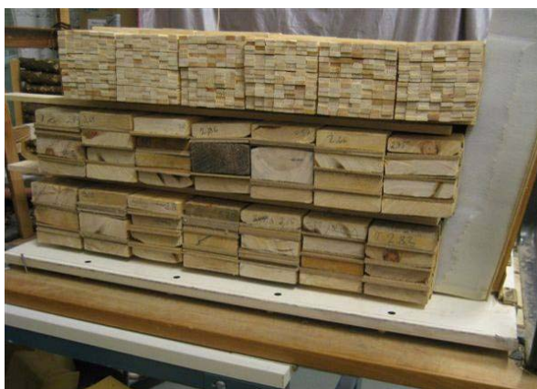
Figure 3.3.6 Force distribution test with three tiers and 6-7 packages in each.
