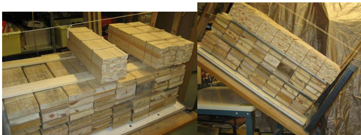
Figure 3.3.1 Wooden slats are placed between the tiers.
