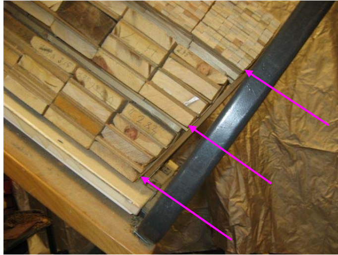
Figure 3.3.2 The tiers of firm packages are seen to push on the uprights with their lower corner, the bottom tier not contributing to the total bending moment on the uprights.
