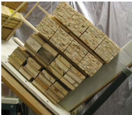
Figure 3.3.4 Force distribution test with four tiers and four packages in each.
