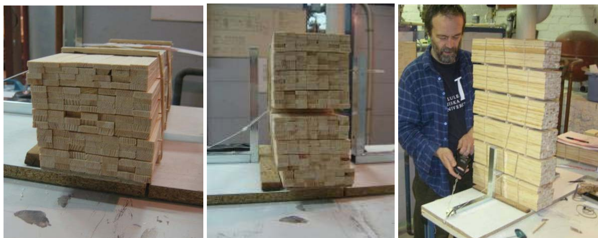
Figure 3.4.10 determination of racking strength as a function of added super positioned weight.
