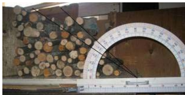
Test nr 5: The slide angle is 45^\circ to 55^\circ from the vertical line.
