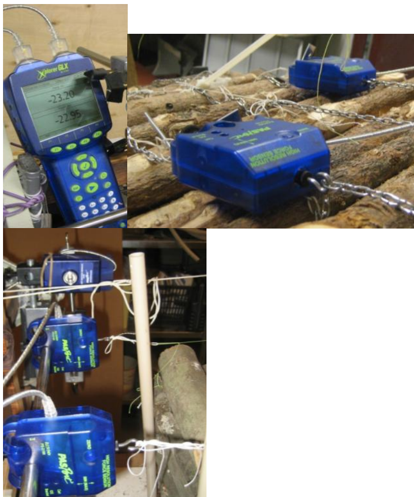
Figure 2.2. (a) The GLX-data logger, (b) Two force sensors attached to top-over lashings and (c) two force sensors measuring the tension in the support wires and a rotary motion sensor.
