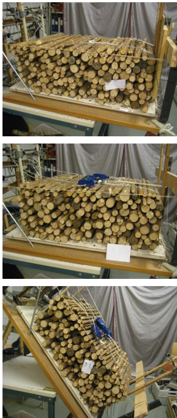
Figure 5.3. (a) The 35 kg stow loaded with procedure II. (b) Blockings removed and top-over lashings tightened. (c) Inclination test 91 under way.
