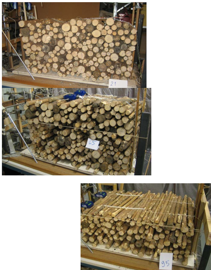
Figure 2.3. (a) the 53 kg stow (test run 31), (b) the 61 kg stow (test run 65) and the (c) 35 kg stow (test run 95).
