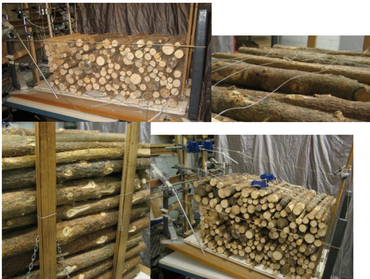
Figure 5.11. (a), (b) The intermediate hog lashings were laid at roughly \frac{3}{4} of the height (c), (d) The top layers of logs were reloaded, top-over lashings set and experiments started.
